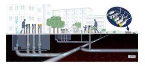
Automated Waste Collection System – Conceptual Diagram In the city's automated waste collection system, garbage inlets connected to underground spaces are installed at various locations, such as apartment buildings and residential courtyards. Sorted garbage is transferred regularly to a waste processing plant via underground pipelines by computer control. Source: City of Stockholm
