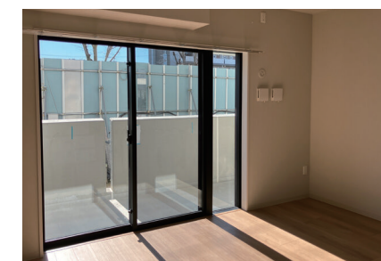
▲ Aluminum-resin composite window frame and double-glazed low-E glass
