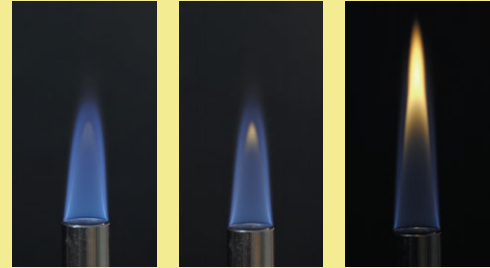
excess air optimum insufficient air
